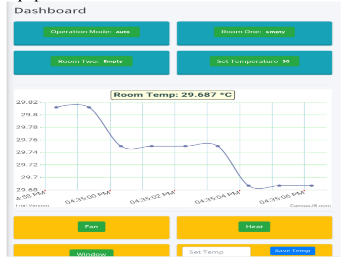
Fig. 2: A picture of the dashboard for the designed smart air conditioner android app.
